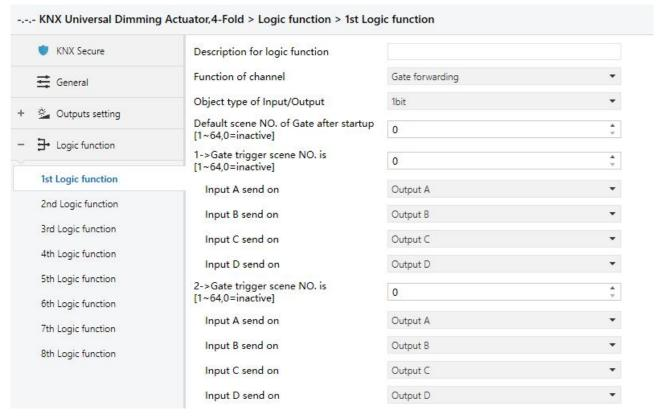
Fig. 5.4.2 "Gate forwarding" parameter window
