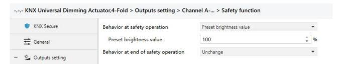
Fig.5.3.3.5 "Safety function" parameter window
