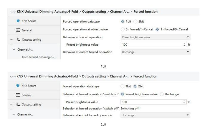
Fig. 5.3.3.4 "Forced function" parameter window
