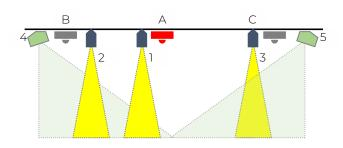
In the figure above the sensors A, B, C regulate the lamps 1,2,3 respectively. A second channel of sensor A regulates lamps 4 and 5, which must both remain on as long as presence is detected by one of the 3 sensors (A or B or C). The second channel of sensor A considers the telegrams of remote sensors B and C.
