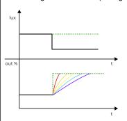
When there is a sudden change in illuminance (in the example the lux is reduced) the system reacts by increasing the control value%, the red slope corresponds to the "very fast" algorithm, the purple one (softer) corresponds the "very slow" algorithm.
