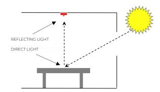
The calibration is to make the value of reflected light as similar as possible to direct light.
