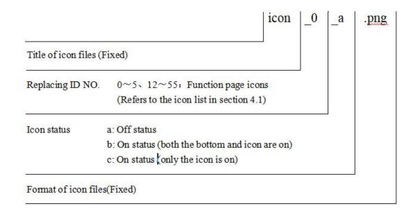
According to the naming rule in the figure above, for examples, icon in the Fig.4.8 is the default icon of which replacing ID number is 0, "icon\_0\_a.png" is off status icon, "icon\_0\_b.png" and "icon\_0\_c.png"are on status icons.
