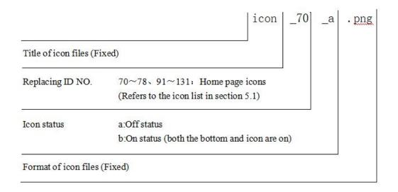
According to the naming rule in the figure above, for examples, icon in the Fig.5.8 is the default icon with replacing ID NO. 70, "icon\_70\_a.png" is off status icon, "icon\_70\_b.png" is on status icons.
