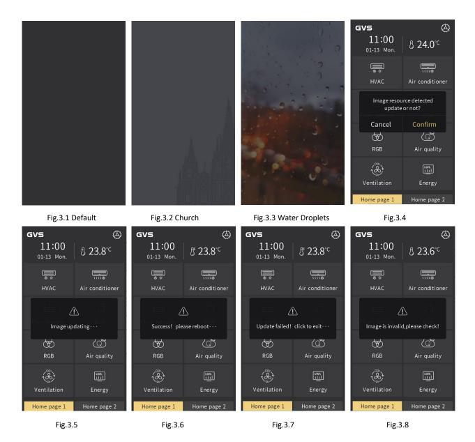
Screen background can be configured as the default background of the system through ETS parameter setting, or insert new pictures via Micro SD card.
