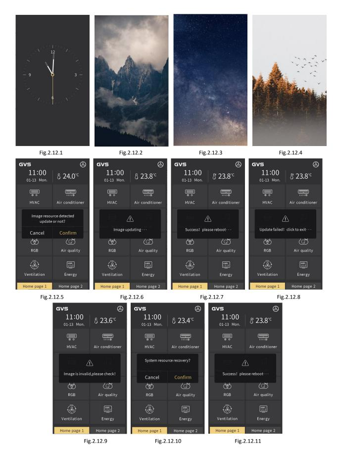
Screen-saver can be set as clock and album that system comes with through ETS parameter configuration, or insert new pictures through Micro SD card.
