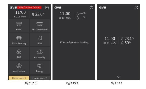
When the KNX bus connection of the device is abnormal, the "KNX Connect Failure" at the top of the interface shown as Fig.2.15.1 above, there is no prompt when the connection is normal.
