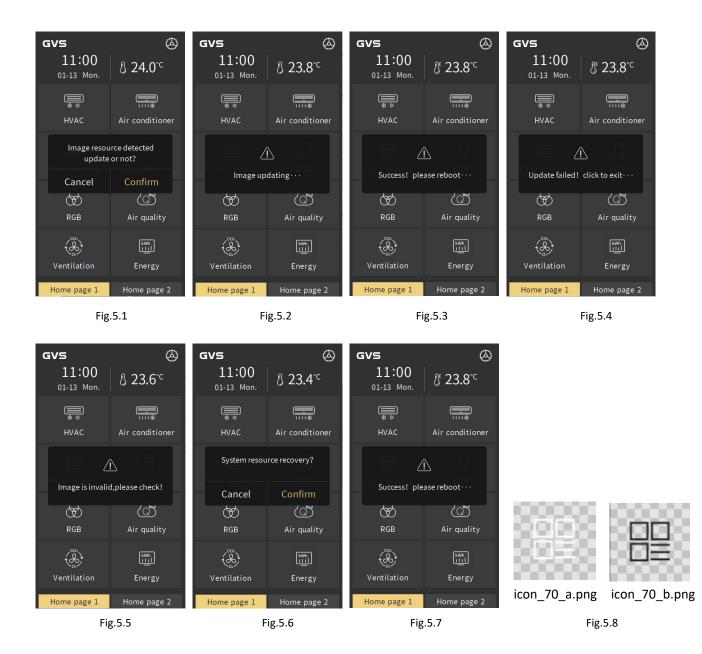
Insert customized icon to replace the original icons of the system through Micro SD card, specific steps as follows:
