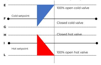
This is used to adjust the opening and closing of the additional valve independently of the speed regulation (for example, once the setpoint has been exceeded, it is possible to perform a maintenance action while still holding the valve open without activating the speeds).
