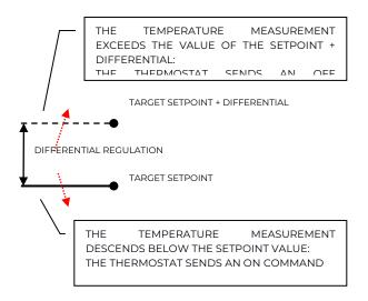
The following image instead shows the operation of the on/off control in cooling.
