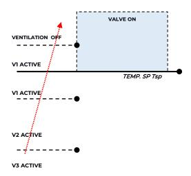
The dashed line area represents the temperature range defined by the "heating regulation differential ON" parameter in case of increasing temperature. When the temperature decreases, the "heating regulation differential ON" parameter defines the valve hysteresis.
