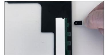
7. Reconnect the keypad control cable and put the glass frame back on the docking station.
