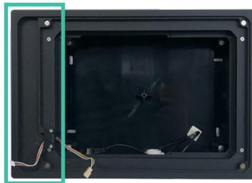
6. Feed the mounting clamps / doglegs through the openings in the corners of the back box and use the included screws and washer to press the clamps tightly against the back of the drywall.
