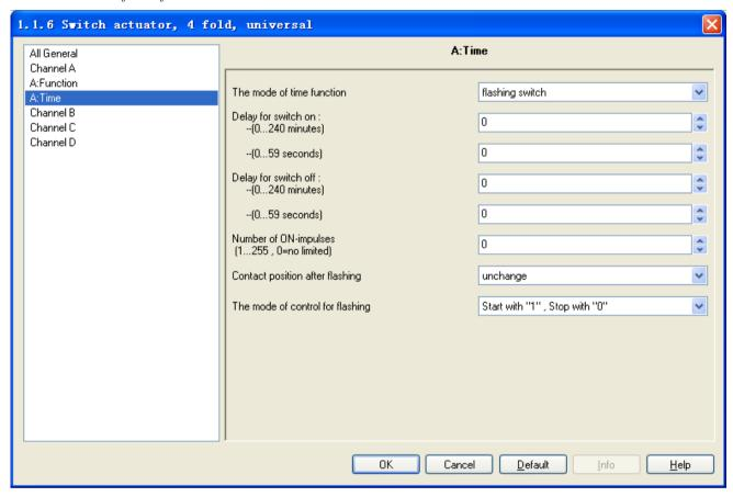
Fig. 2.8 parameter window "X: Time-flashing switch"
