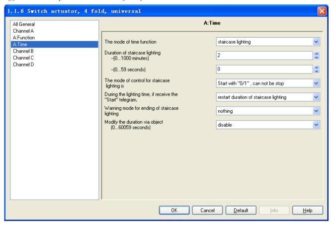
Fig. 2.7 parameter window "X: Time-Staircase lighting"
