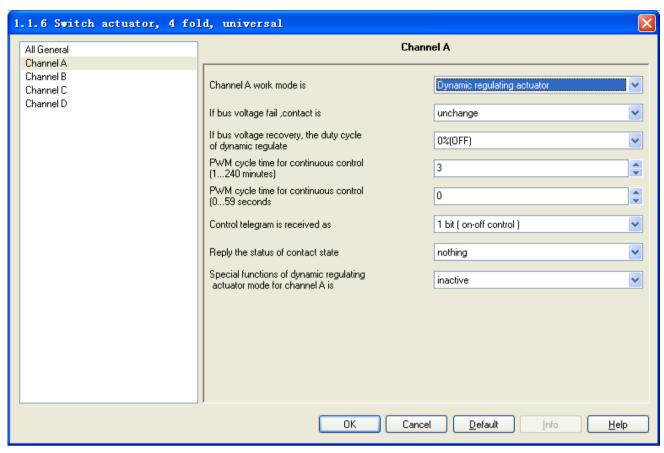
Fig. 2.15 setup window "channel: X-Dynamic regulating Actuator"
