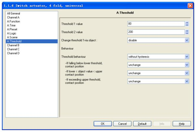
Fig. 2.12 setup window "X: Threshold"
