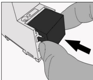
5. Connect the network: The network connections are located on the underside of the device. Connect the IP network cable (RJ45 cable) to the device's network connection (RJ45 pin jack).
