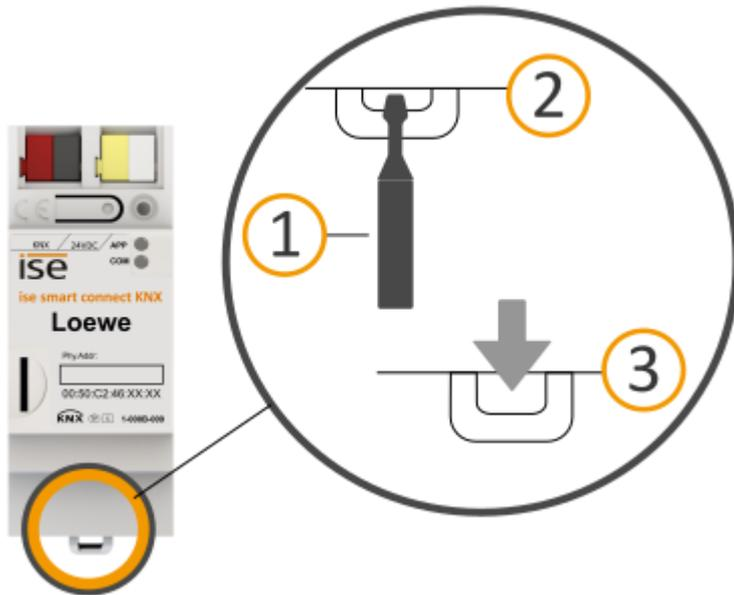
Figure 10: Detach the device from the top-hat rail
