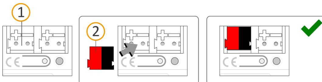
3. Connect the external power supply to the power supply terminal (1) by means of the supplied power connection terminal (2). Polarity: left/yellow: (+), right/white: (-).
