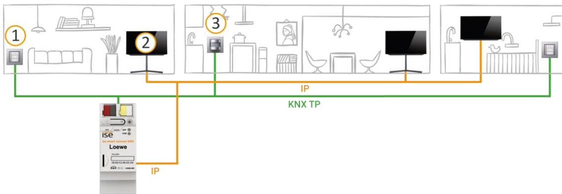
Note: You can control up to two Loewe TV devices with one ISE SMART CONNECT KNX LOEWE.
