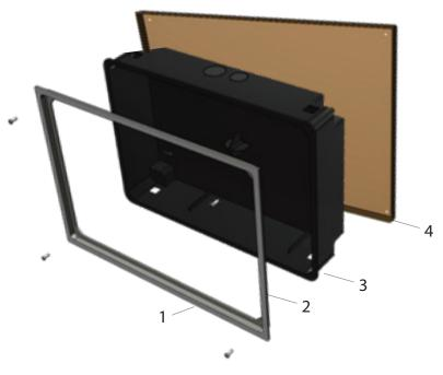
Recess dimensions backbox (W/H/D): 215,0 / 305,0 / 75,0 mm ...... 8.46" / 12.00" / 2.95"
